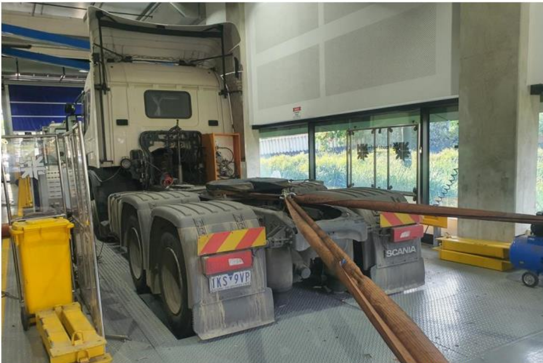
Figure 1. Test vehicle installed on dynamometer
